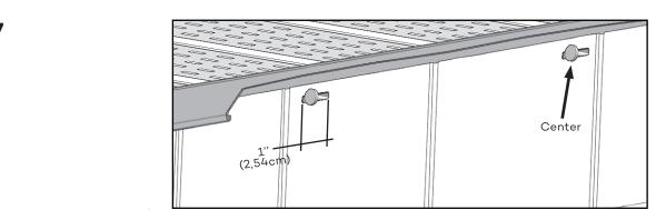
If you need to attach the section in an area other than the installation hole, create a 1"(2,54 cm) long slot to allow nailling. Always nail in the middle of the slot.
