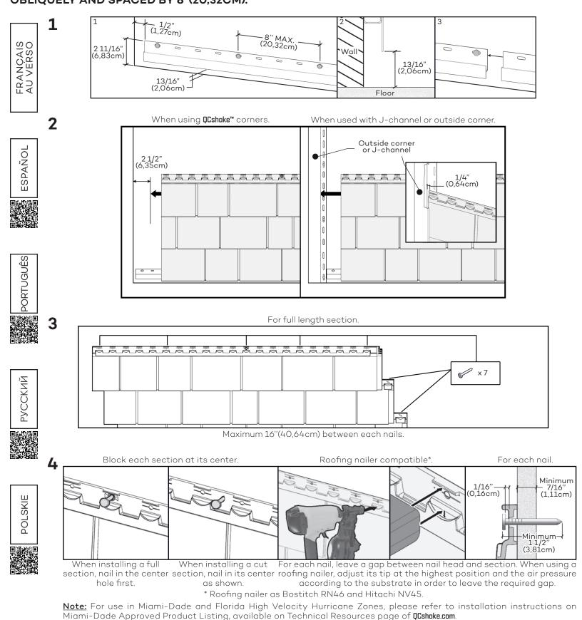
Install sections and space equally. Refer to temperature marks that show the outside temperature the 5 closest to that during installation.
