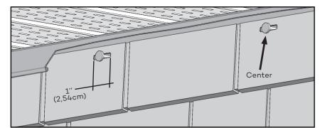
If you need to attach the section in an area other than the installation hole, create a 1"(2,54 cm) long slot to allow nailling. Always nail in the middle of the slot.
