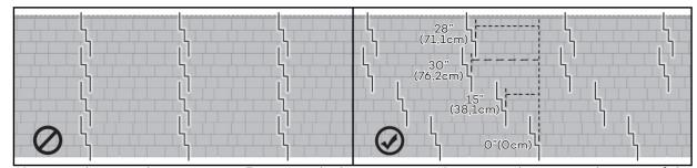
Alternate the joints between rows. For a nicer look, we suggest alternating the cutting distance of the first section of every row from 0"(0cm) - 15"(38,1cm) - 30"(76,2cm) - 28"(71,1cm).
