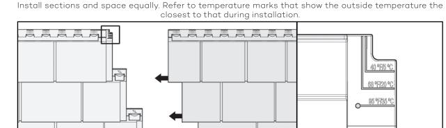
Below 40°F(5°C), position the section slightly right (1/16"(0,16cm)) of the 40°F(5°C) temperature line.
