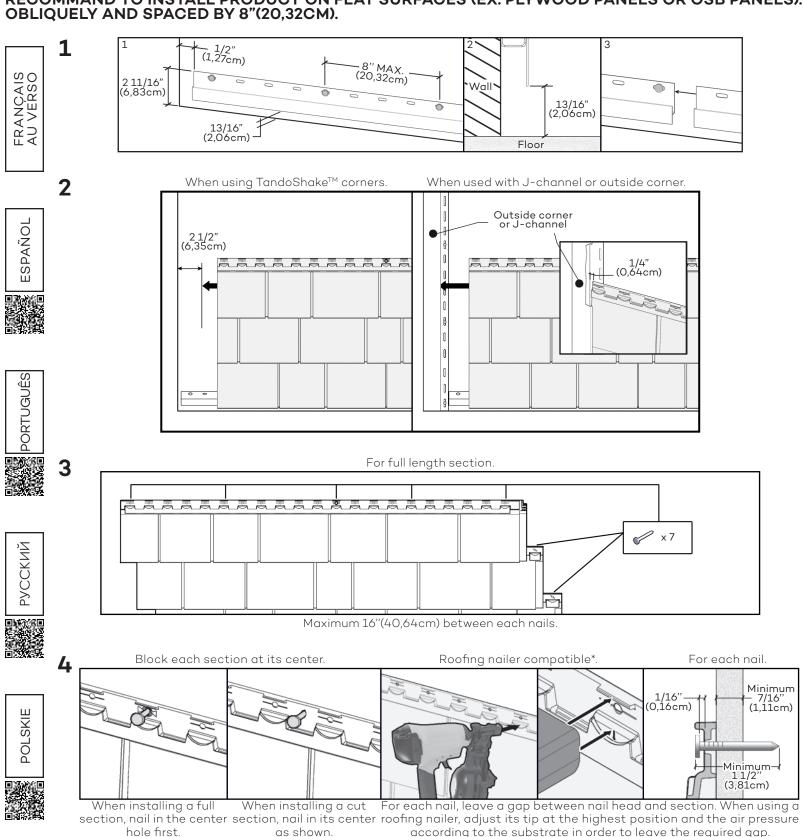
according to the substrate in order to leave the required gap. \* Roofing nailer as Bostitch RN46 and Hitachi NV45.
