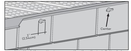
If you need to attach the section in an area other than the installation hole, create a 1"(2,54 cm) long slot to allow nailling. Always nail in the middle of the slot.
