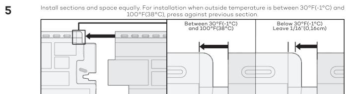
Below 30°F(-1°C), position the section slightly right (1/16"(0,16cm)) previous section.
