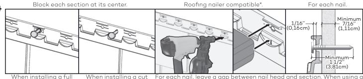
When installing a cut For each nail, leave a gap between nail head and section. When using a section, nail in the center section, nail in its center roofing nailer, adjust its tip at the highest position and the air pressure hole first. according to the substrate in order to leave the required gap. \* Roofing nailer as Bostitch RN46 and Hitachi NV45.
