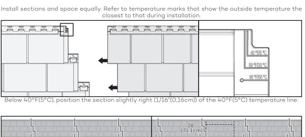
Alternate the joints between rows. For a nicer look, we suggest alternating the cutting distance of the first section of every row from 0"(0cm) - 15"(38,1cm) - 30"(76,2cm) - 28"(71,1cm).
