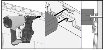
4-Make sure that all pieces are properly joined together (push firmly upwards on the section making sure that the insertion is complete) (Figure 4).
