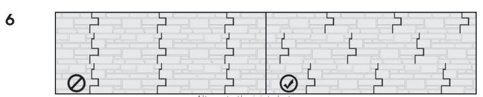
Below 30°F(-1°C), position the section slightly right (1/16"(0,16cm)) previous section.
